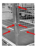
Stop plates, w. shrink flex in middle of both mesh sides/plate sides must be mounted and must afterwards be closed down above the lower trailer sides. See the picture below.
