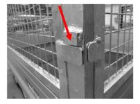
**Check before assembling:** If there are galvanizing residues in the hinge bolts mounting groove or in the mesh side/plate side corner posts mounting groove, these galvanizing residues must be cleaned with grinding tools or chisel before assembling.
