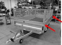
In the case of many demounting and mounting, the self-tapping screws and mesh side/plate side corner posts must be check for wear in connection with the thread for both the self-tapping screws and in the mesh side/plate side corner posts. If there occurs visible wear or that you when tightening the screws feel lack pretension of the screws, the screws and mesh side/plate side corner posts must be replaced.
