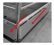
2. Then mount all 4 pcs. mesh side/plate side corner posts to which the mesh side/plate side must be mounted, down into the 4 pcs. lower corner profiles on the trailer. If there are ferrule-end-plugs mounted in the lower corner posts on the trailer, remove these plugs before the mesh side/plate side corner posts can be mounted. See the pictures below.
